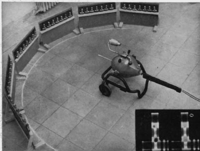
Inspection of the finished parts, in this case the front sight base, uses Gamma Radiography for x-ray inspection.
