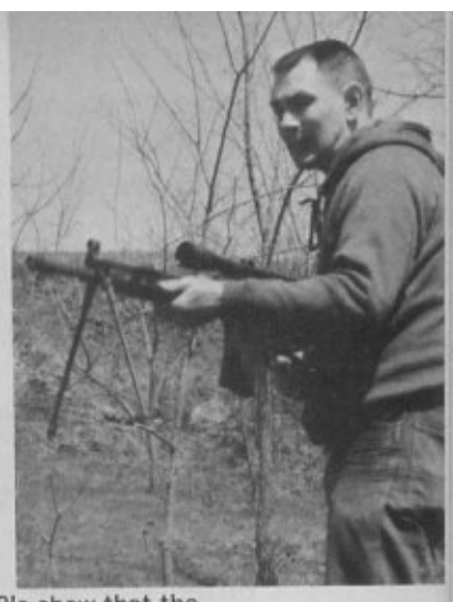
The unfired and fired .308's show that the G-3's chamber leaves flute marks on cases; at right, the CETME's barrel climbs in rapid fire
