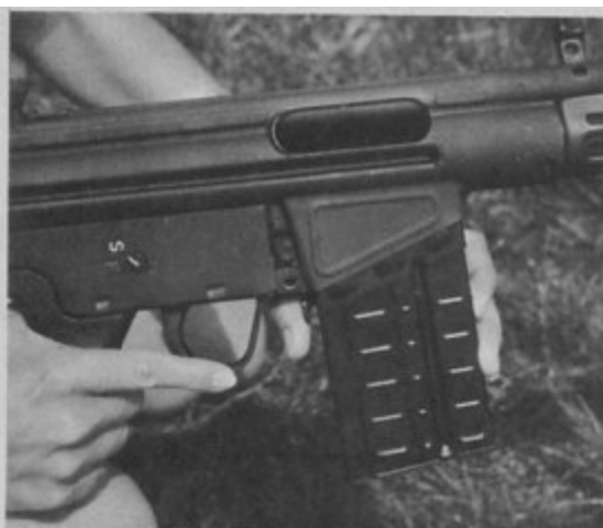
Above, left, the 20-shot clip of the G-3 is released with the left hand, while the right hand remains on the pistol grip. Above right, the 100-yard rear notch is in aiming position and the 400-yard aperture faces you
