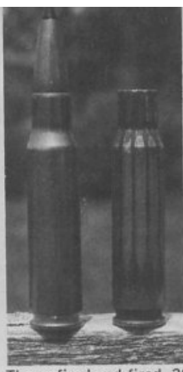
The unfired and fired .308's show that the G-3's chamber leaves flute marks on cases; at right, the CETME's barrel climbs in rapid fire
