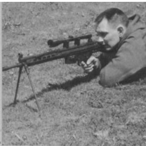
Using the bipod, the author got four-inch groups with the CETME at 100 yards
