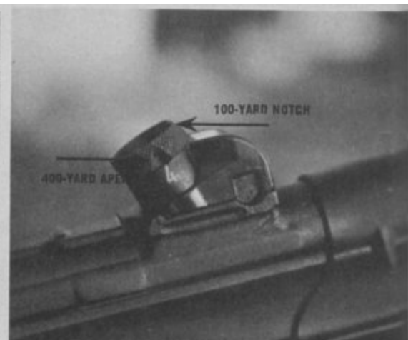
Above, left, the 20-shot clip of the G-3 is released with the left hand, while the right hand remains on the pistol grip. Above right, the 100-yard rear notch is in aiming position and the 400-yard aperture faces you
