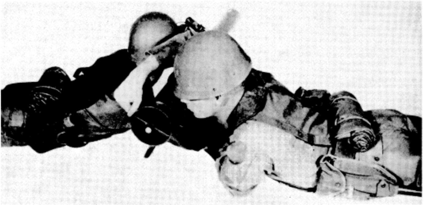
Figure 17. Unlocking and opening the breech.
